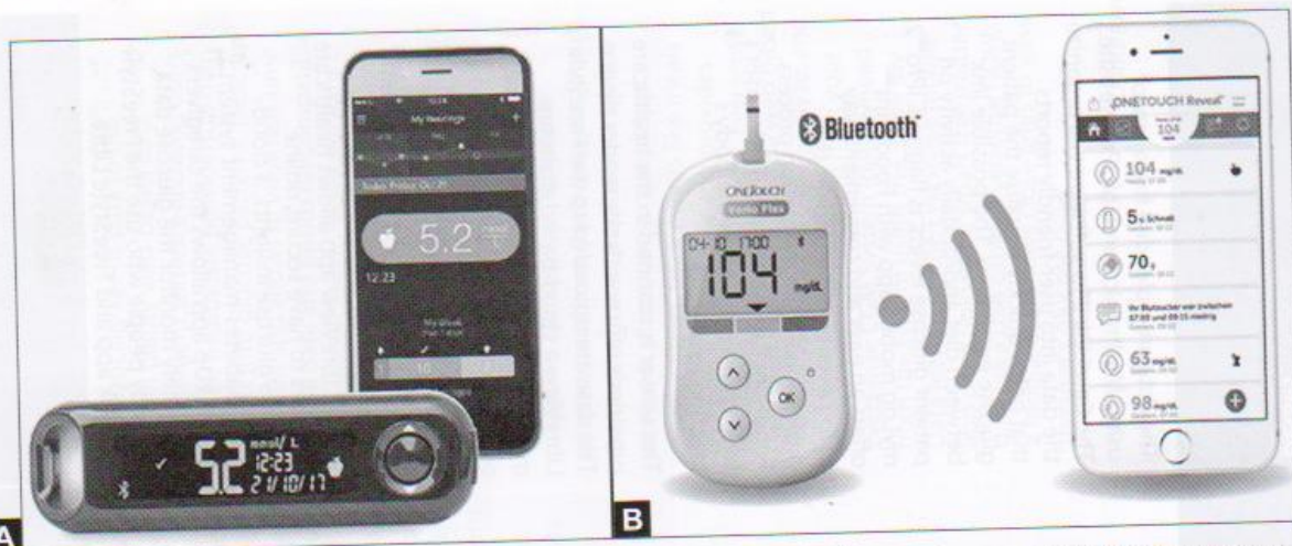
FIGS. 1A AND B: (A) CONTOUR® NEXT ONE blood glucose monitoring system; and (B) OneTouch Verio Flex® blood glucose monitoring system and OneTouch Reveal® application. (For color version, see Plate 6)
