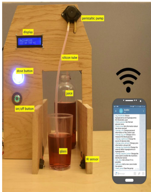
Figure 1: First Prototype, based on communication with Dexcom G4 CGM and the Nightscout solution.
